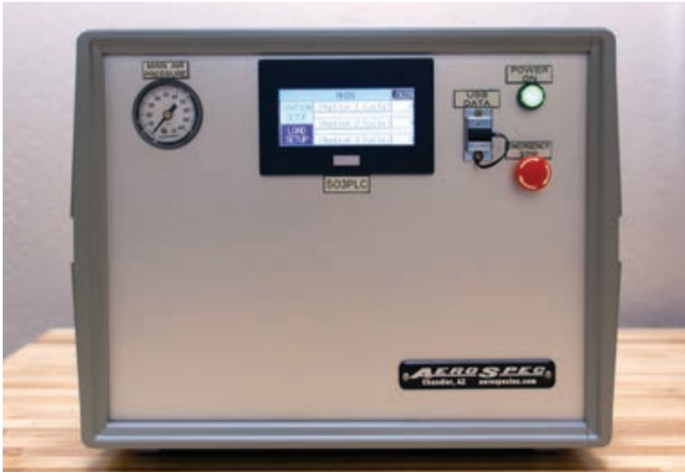
Figure 3: The HMI screen is configured to show all of the test parameters of interest and to guide the operator through the test procedures.
